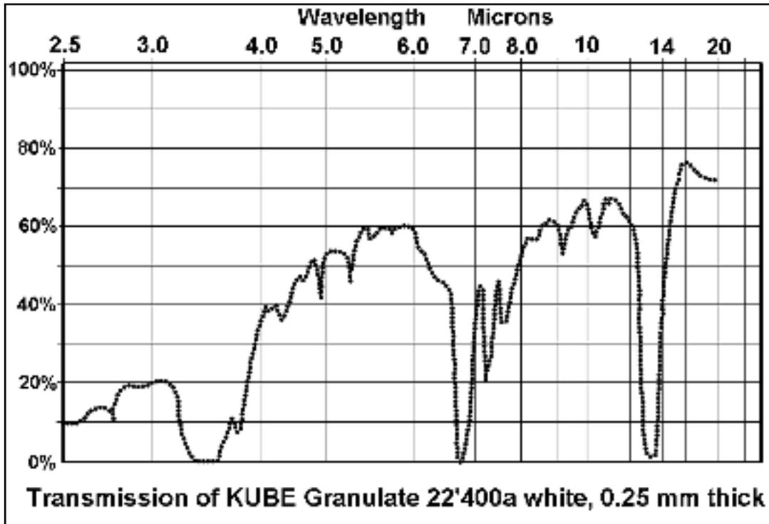
Refractive index at 7...14 microns wavelength is 1.52, optical dispersion is negligible.
