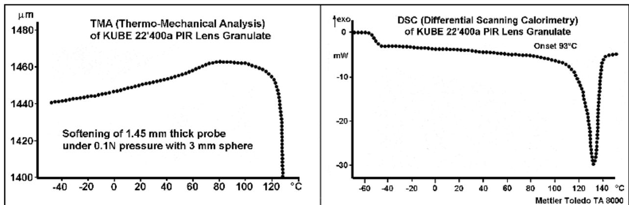
The TMA analysis shows the excellent dimensional stability of KUBE granulates over a wide temperature range. All KUBE PIR plastics can be used over a temperature range of -40 ... +85°C. According to the DSC plot, there are no phase transitions and no glass phase formation within this range.
