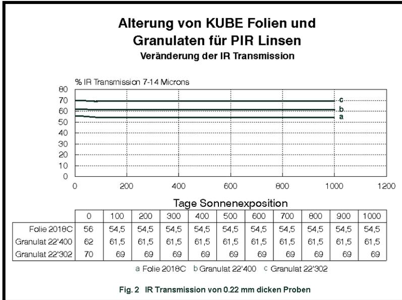
The graph shows the change of infrared transmission over 1000 days for probes of 0.22 mm thickness and various KUBE materials.
