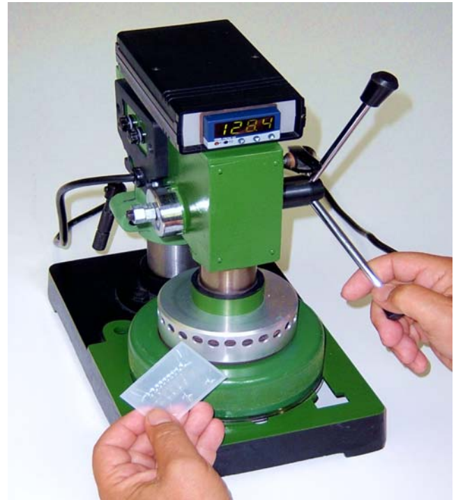
Hot press to make prototype fresnel lenses
